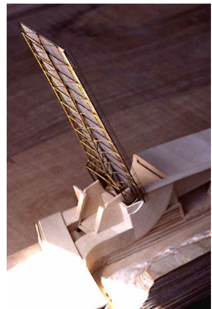
37. Bascular leaf, structural model.
