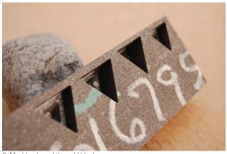
8. Machined graphite mold block
