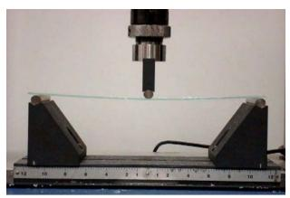
Figure 4: Flexure test - 1/8" annealed glass
