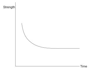
Figure 9: Glass strength and load duration 4
