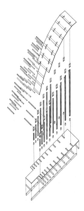
Fig. 3. Stair: exploded axonometric.
