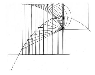
Fig. 1. Stair: motion diagram.
