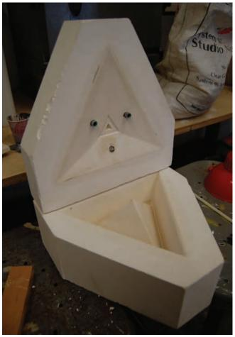
45. Pottery plaster molds for slip casting
