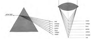
4. Prismatic and lens refraction
