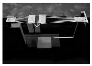
Fig.3 Holleman compression-tension probe.
