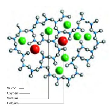
Figure 2: Molecular composite of glass crystal
