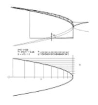
9. Geometric modeling, parabolic construction projected to sectional profile.
