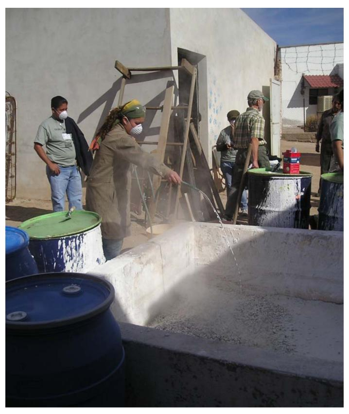
Abby Valenzuela, INAH-Sonora, demonstrates the hydration process of lime plaster production.
