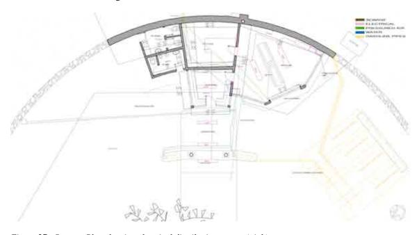
Figure 27 - Systems Plan showing electrical distribution system (pink).
