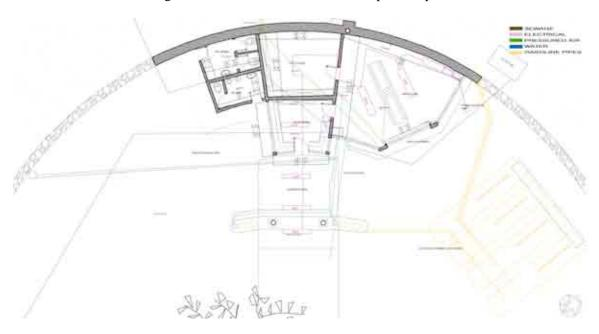
Figure 38 - Systems Plan showing the pressured air distribution system (green).
