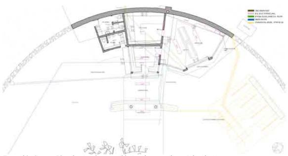
Figure 21 - Systems Plan showing the water (blue) and sewage (brown) distribution systems.
